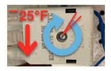
3. The gas oven thermostat is built into the back of this CE gas oven valve body. This valve does not have a temperature calibration adjustment, it is set by the valve manufacturer. In the event that the average oven temperature consistently tests above or below 25°F from set dial temperature, the gas valve should simply be removed and replaced. Please contact our Support Department for replacement parts or further instructions.
