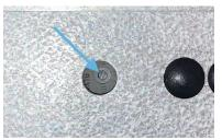
2. To adjust the thermostat you may first need to scrape the anti-tamper paint from the screw head groove. Make certain to use a fine-blade (1/8" wide) screwdriver to avoid stripping the screw. Rotate the screw Clockwise to Decrease temp - about 10 degrees of arc = approx. 25°F of temp adjustment.
