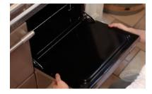
Set the door face-down on a protected work surface and release the spring tension on each upper hook arm using a hand tool as a lever to unlock the arms.
