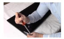
7. Thread the top two inner door panel screws into place, but do not tighten yet. The panel should remain allowed to float slightly to install the gasket. Then thread the original screw hardware to the bottom of the door assembly, but also do not fully tighten yet.
