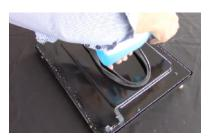
9. Now position the rubber peripheral gasket into the seam making sure to align the notches in the rubber strip over each mounting screw and brass grommet at the bottom of the door. Then press the gasket straight down into the seam at each screw and grommet taking care not to stretch the rubber in either direction.
