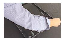
11. Then press the gasket into the seam all around the door without pulling or pushing the rubber laterally along the seam, or else it will bunch up in spots. Continue until the entire depth of the rubber gasket is pressed fully into the seam up to the edge of the outer door panel flange.
