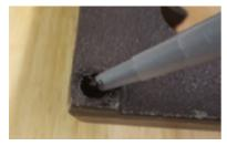
4. Using a toothpick or a straightened paperclip "rod", insert the rubber grate foot past the side of the rod to allow any air and/or excess RTV Silicone to squeeze out of the socket from underneath the rubber foot. Then remove the rod and clean up any excess RTV with a spare rag or towel.
