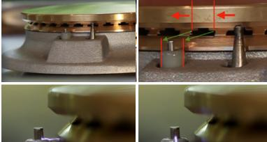
3. To adjust the height of the spark electrode: Remove the burner cap & base, then gently pull up on the electrode, use your free index finger to rotate the brass nut at the base of the spark electrode (Clockwise to raise the electrode & counter-clockwise to lower the electrode).
