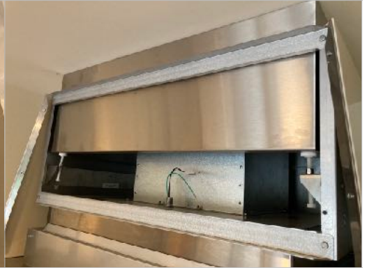
27. Reinstall the front panel support bracket(s). Make sure the bracket fixes the body side panels as wide as possible at the top.
