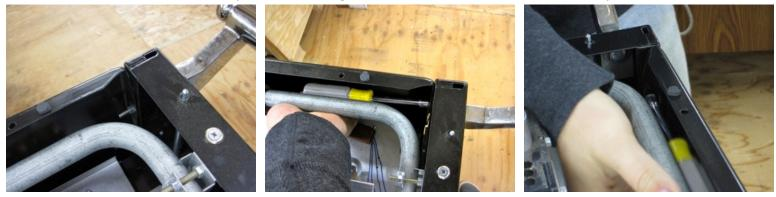
3. Remove the phillips screws along the top of the control panel and all the handle knobs across the front.
