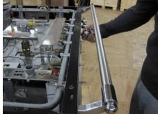
Remove the control panel ground strap [if applicable] and pull the control panel straight off the front. Take care not to damage the LED wires, label and unplug the LED connections. The control panel is now free to remove.
