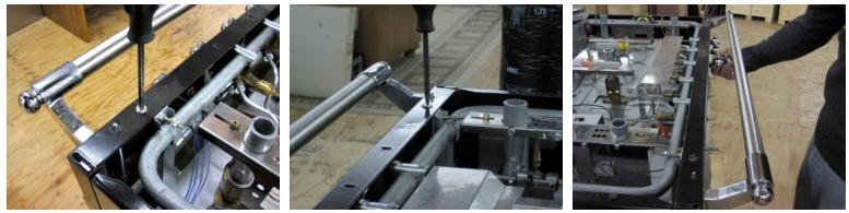
4. Remove the control panel ground strap [if applicable] and pull the control panel straight off the front. Take care not to damage the LED wires, label and unplug the LED connections. The control panel is now free to remove.
