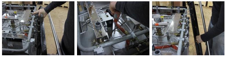
5. The control panel venting flange slides just under the flashing located under the valves when reinstalling the control panel. Mind the oven control shafts when reinstalling. Install in reverse order.
