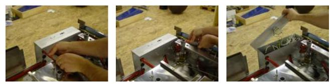
5. Remove both 7mm screws at each side. These screws are installed from the rear. These will be difficult to remove considering the back panel will be close to the wall. If a 7mm nutdriver is too long, consider using a 7mm open end wrench or socket to loosen the screws.
