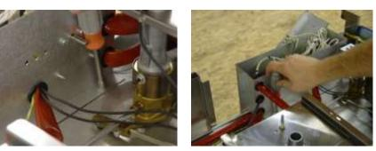
7. Electrical box front is free to move, angle it forward while shifting it to the side.
