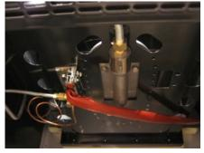
5. With an 8mm nutdriver, loosen the locking nut to unlock the 2mm Allen set screw. Now loosen the 2mm set screw to release the air collar. Slide the air collar back far enough to access the main burner injector. Remove and replace the main burner injector with a 12mm wrench. Use the new washer supplied with the new injector.
