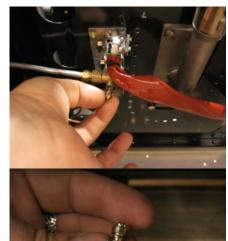
7. Be sure to re-adjust the main burner air collar to the proper gap opening\* and tighten/lock the 2mm set screw:
