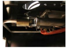
6. With a flathead screwdriver, remove the cap screw at the bottom of the pilot assembly. Next, carefully remove the pilot injector and replace with the new one (NAT=0.45mm, LP=0.25mm). When installing the new pilot injector, tighten against the spring load until you clearly feel the injector bottom out. This is the standard adjustment for the needle valve.
