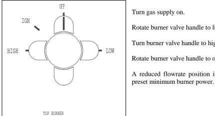
Turn gas supply on.Rotate burner valve handle to lighting position.Turn burner valve handle to high position for maximum flame.Rotate burner valve handle to off position.A reduced flowrate position identified by the "Low" mark produces the
