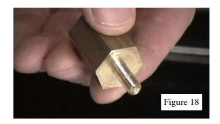
**Note:** Over-tightening the brass coupler adapter could fracture the enamel on the front panel. (Figure 19)
