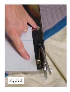
3. Remove the two or three screws from the bottom of the oven door. (Figure 6)
