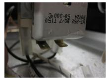
2. Check continuity between the spade connections on the thermostat during entire temperature range. Replace as necessary (refer to Retaining clip on step 4).
