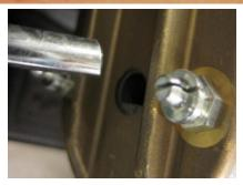
5. Make sure the gas oven selector switch is properly seated and secure to the main gas oven valve body. This simply clips into place.
