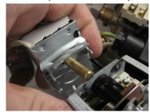
4. Make sure the gas oven thermostat is properly seated to the selector switch via the retaining clip.
