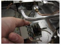
3. Remove the selector switch/thermostat unit simply by pulling straight toward the back of the valve body. Check continuity on gas oven selector switch terminal connections. Replace as necessary.
