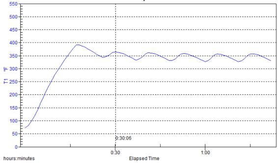
The example above is an actual plot line graph featuring the REAL-TIME temperature reading on a Lacanche Cluny electric oven set to 350°F.
