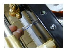
Shove the metal bezel through the hole. If the hole seems too small or tight, push on the bezel firmly while making a circular motion with your thumb, causing the bezel to gyrate. This should open the hole and allow the LED to insert into the hole.
