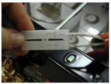
3. Remove the old LED by pushing it through the control panel from the rear. Thread the LED + wires into the broad end of the metal bezel and snap it into place (until the lens is flush). Attach the mini insulator clips on the LED wire ends and then thread both wires through the hole in the control panel one at a time.
