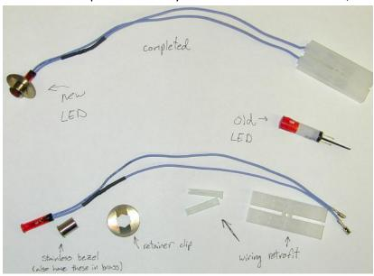
Be sure to replace one LED at a time as not to confuse the location of each LED. Remove each wire connector from the back of the old LED. You will need to remove the plastic clip from the ends of each wire by prying open the clip with a small flathead screwdriver and pulling the clip off the spade connector.
