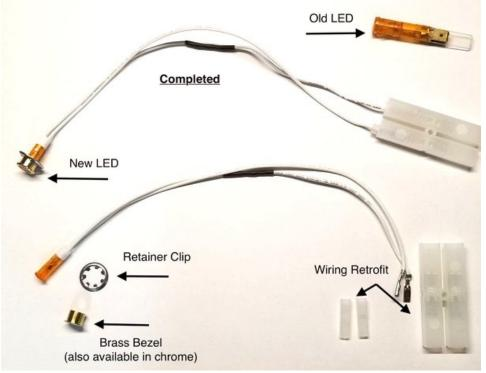
Carefully remove each wire connector from the back of the old LED. You will need to remove the plastic insulator from the ends of each wire by prying open the clip with a small flathead screwdriver (or pinching the exterior of the plastic insulator with a pair of pliers near the internal tab clip) then pull the insulator off the spade connector.
