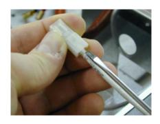
Next, insert each spade connector into the clear plastic wiring coupler like shown.
