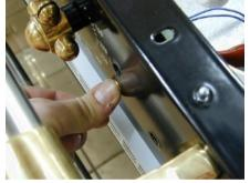
5. Thread the wire ends through the circular retainer clip with the teeth on the clip pointed towards the wire ends like shown. While backstopping the front of the LED lens to firmly hold it against the control panel surface, incrementally slide the retainer clip over the bezel until firmly seated to the control panel.
