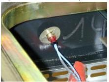
6. Place the LED wire ends into the Heyco connector and seat them fully into place using a thin blunt tool like the end of a screwdriver. Note: Since polarity is not an issue, the position of each LED wire can be positioned in either side of the connector.
