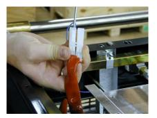
Pull the silicone sheathing over the wire coupler and repeat this process on remaining LED's.
