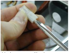
2. Insert each spade connector into the clear plastic Heyco H-block connector like shown.
