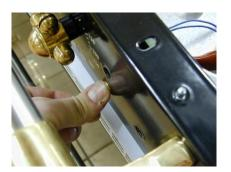
Thread the wire ends through the duckbill retainer clip with the cutouts on the clip pointed towards the wire ends like shown. While pushing on the front of the LED, slide the duckbill clip over the bezel until firmly seated.
