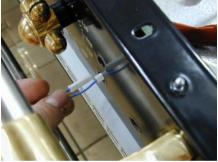
4. Shove the metal bezel through the hole. If the hole seems too small or tight, push on the bezel firmly while making a circular motion with your thumb, causing the bezel to gyrate. This should slowly enlarge the hole by gently scraping enamel material from the inside edge of the hole to allow the LED bezel to be fully inserted.
