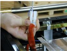
7. Pull the silicone sheathing over the Heyco connector and repeat this process on the remaining LEDs.
