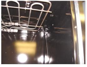
Now remove each black clip by pinching to release the spring tension while pulling down on the clip. You may need to rock it back and forth while pulling down to draw it from the hole in the oven ceiling.
