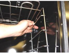
Maneuver this probe out of the two black spring clips and let it hang from the rear of the oven. You may want to remove the oven rack guide and thumb screw just below this probe to give you more room to work.
