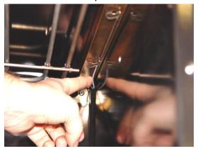
This is how the thermostat probe and heat shield should look when successfully installed.
