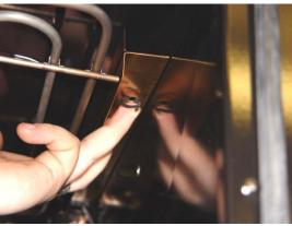
Now re-install the thermostat probe into each clip. Make sure this probe is pinched and held between the "fingers" of the black clips. If the clips are not able to hold the probe, then make it rest at a position furthest away from the oven element while in the clip.
