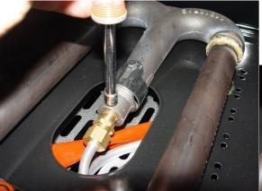
With a 7mm nutdriver, loosen the locking screw to remove the injector assembly from the gas oven burner. Remove the injector using a 12mm and 16mm wrench.
