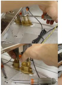
With a 7mm nutdriver, loosen the air collar and shift it up out of the way to get to the injector. Remove the injector with a 12mm wrench. Use the new washer supplied with the new injector.
