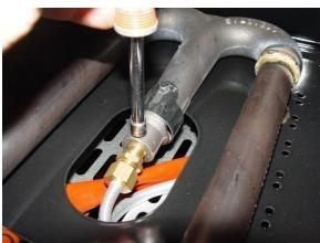
With a 7mm nutdriver, loosen the locking screw to remove the injector assembly from the gas oven burner. Remove the injector using a 12mm and 16mm wrench.
