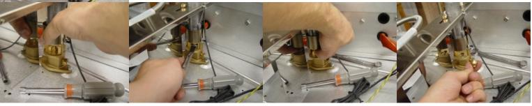
Now adjust the air collar and low flame adjustment for each burner by viewing the "Air Collar Adjustment" video and the "Burner Flame Adjustment" video found at:
