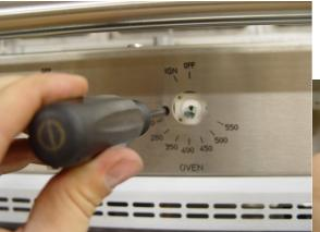
With a flathead screwdriver, turn the selector screw counterclockwise all the way to the stop, labeled "N" for Natural Gas or clockwise to the stop, labeled "LP" for Liquid Propane.
