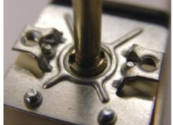
3. Use the adjustment tool supplied by Art Culinaire or a pair of needle-nose pliers to adjust the slip collar.
