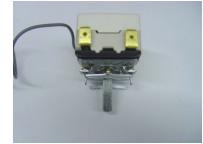
2. Now pull the T-stat straight off the back of the switch to expose the T-stat shaft and slip collar.
