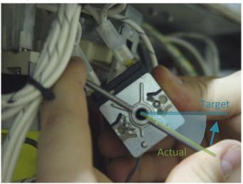
You will be adjusting the threaded slip collar against the threaded D-shaft on the T-stat. Ultimately changing the physical position of the D-shaft on its long axis. Be sure to make your adjustment in the opposite direction of the dial temperature markings. Clockwise to lower target temperature, counter-clockwise raise target temperature.
