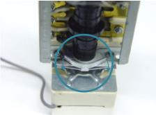
Conversely, the retainer clip holds onto the T-stat by interlocking these two tabs (one is bent at a sharper angle than the other) into screw holes on the T-stat. This only installs one way, left side first, looking at the back plate with the wires at the top.
