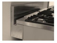
After the brackets are installed correctly, pull the range away from the wall and drop the back lip of the wall spacer over the brackets. Push the range up to the back spacer.
