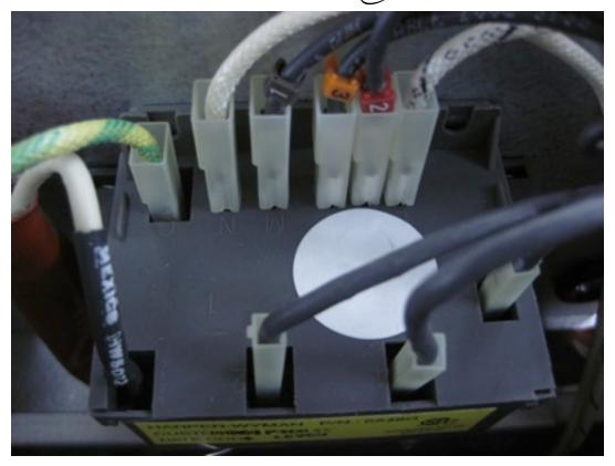
HARPER-WYMAN P/N: 6548G - Art Culinaire P/N: 65.226005-3+1 Input: (120v 60hz 4mA)
